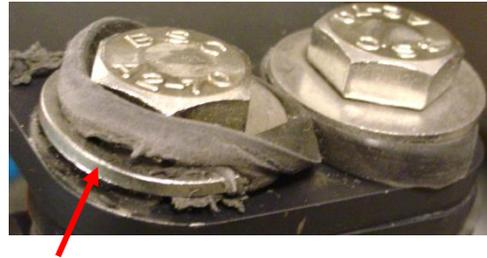
Figure 4: Sharp Edge of the Washer Against the Shock Isolator
