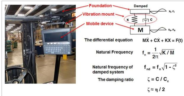
Figure 2: Typical Vehicle Computer Installation with Isolation Mounts
