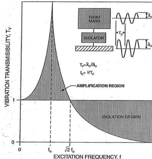
**Figure 1: Qualitative Representation of Vibration Transmissibility for an Undamped Linear Isolation System**
